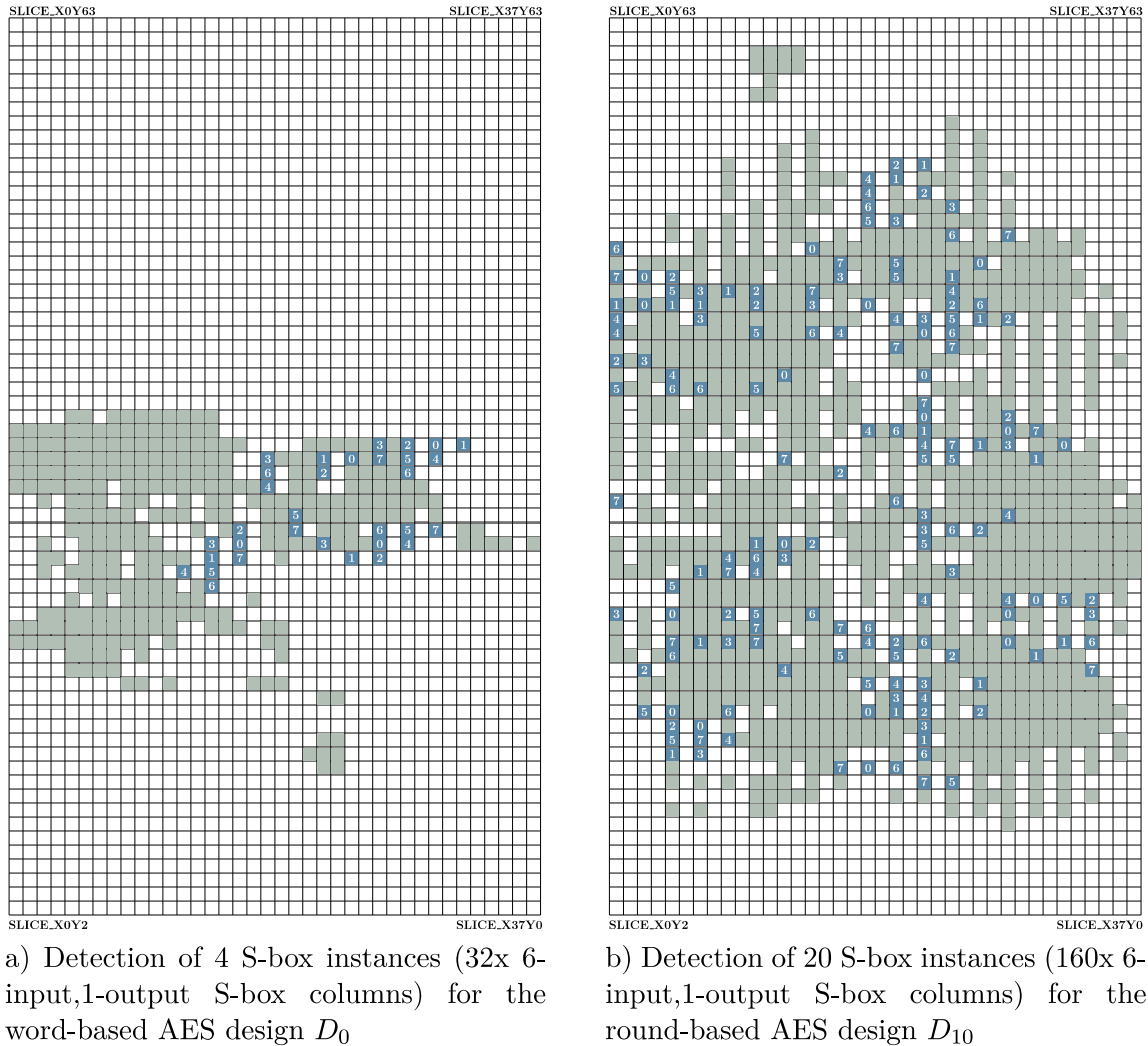
Figure 4.7: FPGA grid view of a Xilinx Spartan 6 XC6SLX16, where each cell represents one slice. It shows the results of the proposed 8-input, 8-output S-box detection algorithm for AES hardware configurations. Any cell containing a number shows that the i^{th} (with i \in \{0, 1, \dots, 7\} ) AES S-box output column is implemented by the corresponding slice, i.e., it is successfully detected. White cells represent unused slices, whereas gray cells denote the usage of arbitrary combinatorial logic within one slice, i.e., at least one out of 4 LUTs is configured
