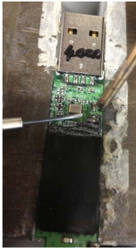
Figure 5.2: Epoxy removal of Kingston DT 5000 with screwdriver
