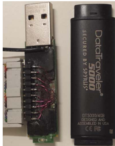
Figure 5.3: Eavesdropping the bitstream of Kingston DT 5000 with opened case
