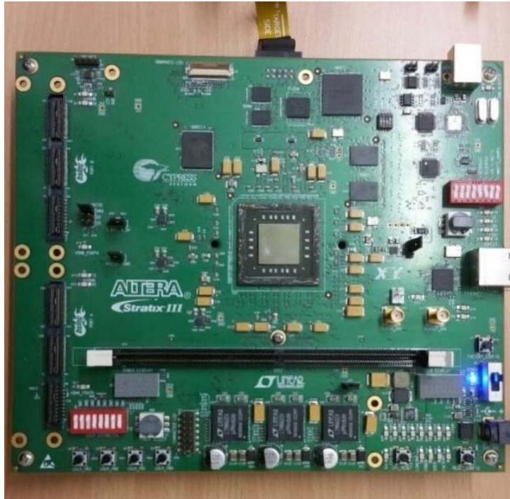
Figure 3.1: Device under attack - Official development board containing a Stratix III FPGA
